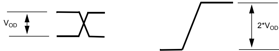
Figure 19 - Differential Voltage Parameter
