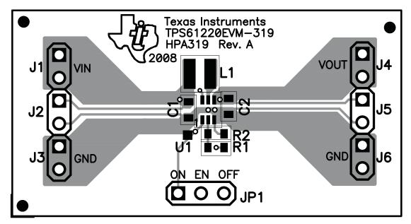
Figure 1. Top Assembly Layer
