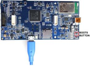
Figure 6. Micro USB Connection and BOOTO Button Used when Upgrading Firmware
