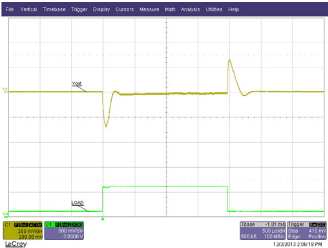
Figure 3. Typical Transient Load Response for a 100mA to 600mA Transient Load V_{IN} = 3.5V
