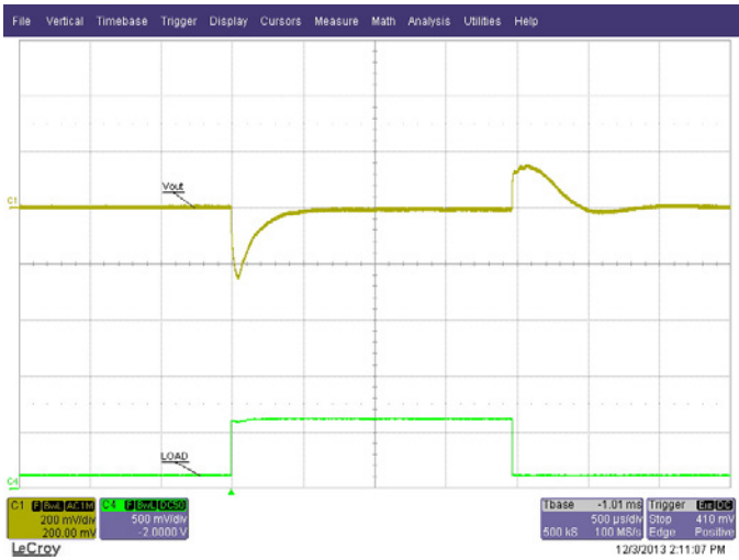
Figure 4. Typical Transient Load Response for a 100mA to 600mA Transient Load V_{IN} = 12V
