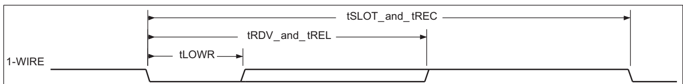
Figure 6-60. 1-Wire Read Bit Timing (Data)
