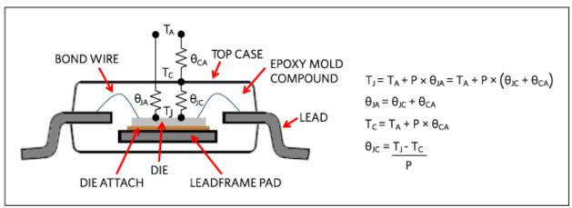
Figure 1. An industry-standard thermal model and formulas for integrated circuit devices.
