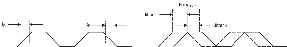
Figure 1. SMAART wire™ / UART Interface Timing Diagram
