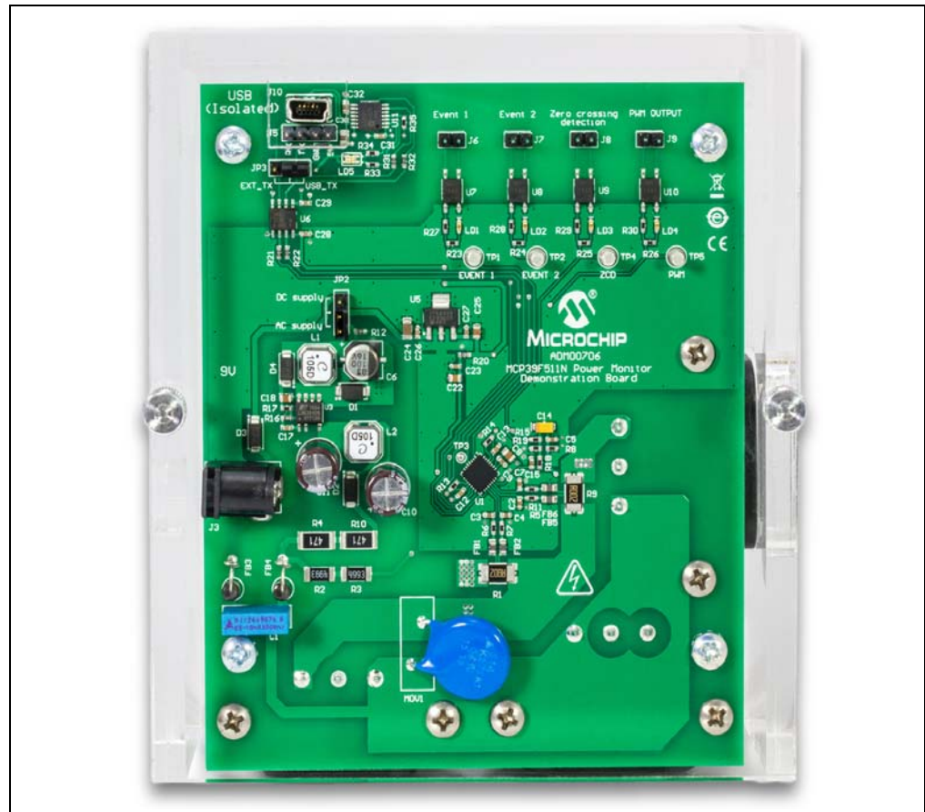
FIGURE 1-1: MCP39F511N Power Monitor Demonstration Board.
