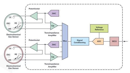
Figure 2. Dual-channel integrated gas sensing signal chain (simplified).
