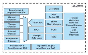
Figure 5. Simplified functional block diagram of the ADuCM355.
