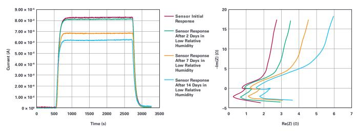
Figure 3. The correlation between sensor sensitivity (left graph) and impedance (right graph) during accelerated lifetime test in low relative humidity.
