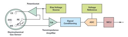
Figure 1. Typical electrochemical gas sensor signal chain (simplified).
