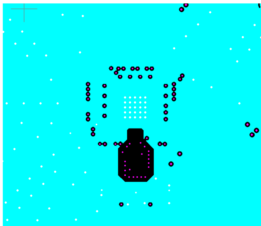
Figure 11.8. Bottom Layer Ground Flooded (Layer 3)
