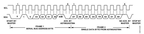
Figure 29. Reading a Single Byte of Data from a Selected Register
