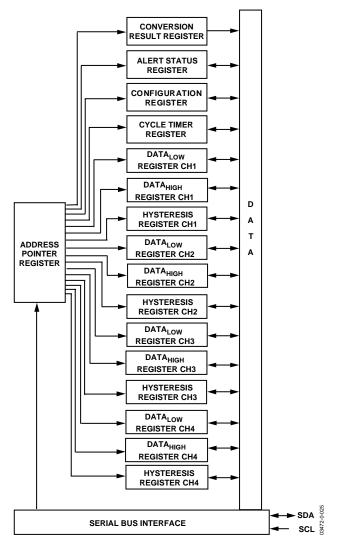
Figure 25. AD7993/AD7994 Register Structure
