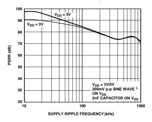
Figure 6. PSRR vs. Supply Ripple Frequency
