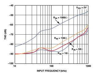
Figure 24. THD vs. Analog Input Frequency for Various Source Impedances for  $V_{DD} = 5 V$ , 136 kSPS, Mode 1
