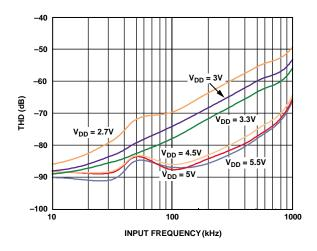
Figure 23. THD vs. Analog Input Frequency for Various Supply Voltages,  $F_S = 136$  kSPS, Mode 1
