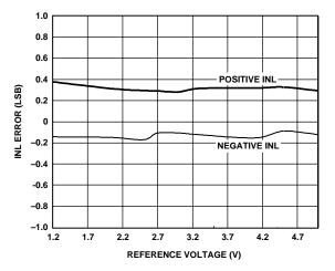
Figure 12. AD7994 Change in INL vs. Reference Voltage  $V_{\rm DD}$  = 5 V, Mode 1, 121 kSPS
