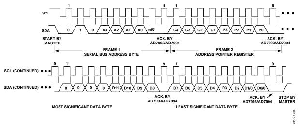
Figure 28. Two-Byte Write Sequence
