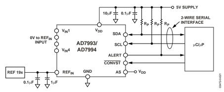
Figure 22. AD7993/AD7994 Typical Connection Diagram
