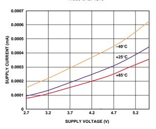
Figure 14. AD7994 Shutdown Current vs. Supply Voltage,  $-40^{\circ}$ C,  $+25^{\circ}$ C, and  $+85^{\circ}$ C
