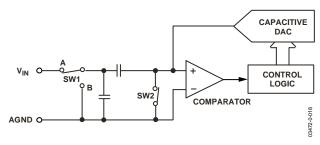
Figure 18. ADC Acquisition Phase
