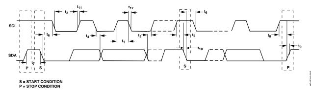
Figure 2. Two-Wire Serial Interface Timing Diagram
