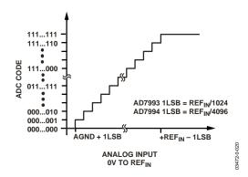
Figure 20. AD7993/AD7994 Transfer Characteristic
