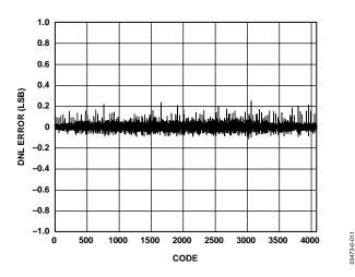
Figure 11. AD7994 Typical DNL,  $V_{DD}$  = 2.7 V, Mode 1, 3.4 MHz  $f_{SCL}$ , 121 kSPS
