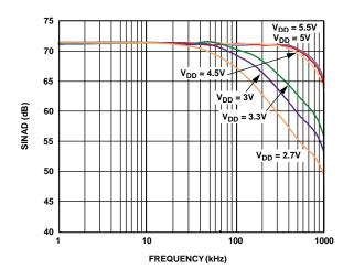
Figure 7. AD7994 SINAD vs. Analog Input Frequency for Various Supply Voltages, 3.4 MHz f<sub>SCL</sub>, 136 kSPS
