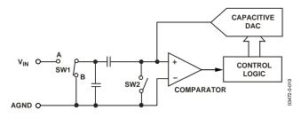
Figure 19. ADC Conversion Phase
