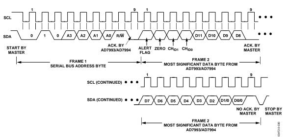
Figure 30. Reading Two Bytes of Data from the Conversion Result Register
