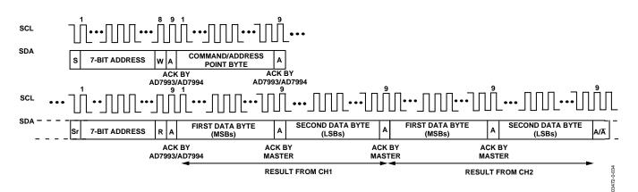
Figure 34. Mode 2 Sequence Operation
