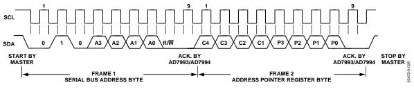
Figure 26. Writing to the Address Pointer Register to Select a Register for a Subsequent Read Operation
