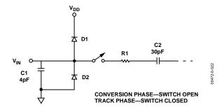
Figure 21. Equivalent Analog Input Circuit
