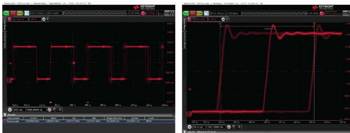
Figure 6. High frequency jitter on recovered clock (RCLK) when frequency difference between G.703 and MCLK is greater than 1Hz.
