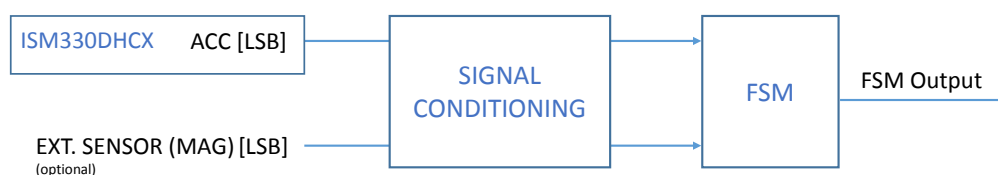
Figure 2. State machine in the ISM330DHCX
