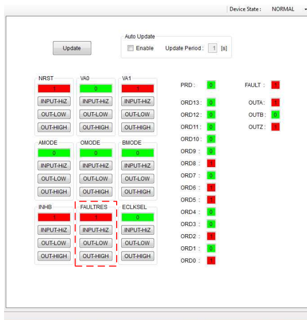
Figure 16. FAULTRES Change in Pin Configuration Tab
