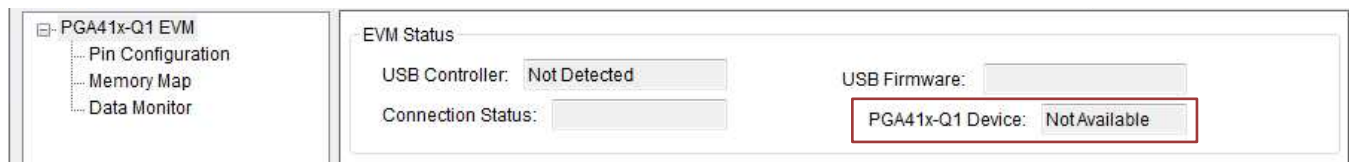
Figure 4. PGA411-Q1 Device Startup Failed
