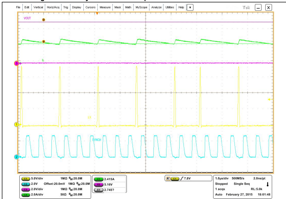
Figure 23. Valley current sense operation in overcurrent condition
