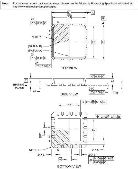
24-Lead Very Thin Plastic Quad Flat, No Lead Package (MJ) - 4x4 mm Body [VQFN] Punch Singulated; With 2.5x2.5 Exposed Pad
