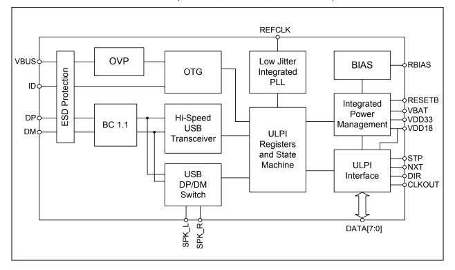
FIGURE 1-1: BLOCK DIAGRAM (USB3341, USB3346, AND USB3347)
