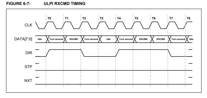
Transfer of the RXCMD byte occurs in Synchronous Mode when the PHY has control of the bus. The ULPI Protocol Block shown in Figure 6-1 determines when to send an RXCMD. A RXCMD will occur:
