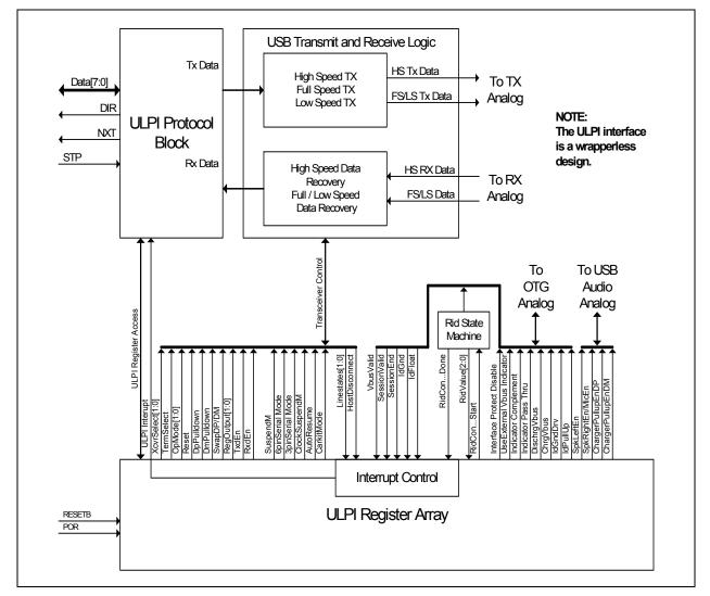
FIGURE 6-1: ULPI DIGITAL BLOCK DIAGRAM
