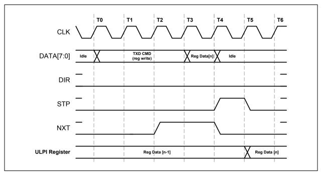
To write a register, the Link will wait until **DIR** is low, and at T0, drive the TX CMD on the data bus. At T2 the PHY will drive **NXT** high. On the next rising clock edge, T3, the Link will write the register data. At T4, the PHY will accept the register data and drive **NXT** low. The Link will drive an Idle on the bus and drive **STP** high to signal the end of the data packet. Finally, at T5, the PHY will latch the data into the register and the Link will pull **STP** low.
