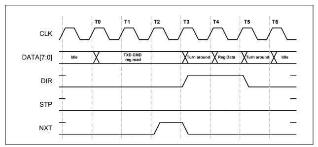
FIGURE 6-5: ULPI REGISTER READ IN SYNCHRONOUS MODE
