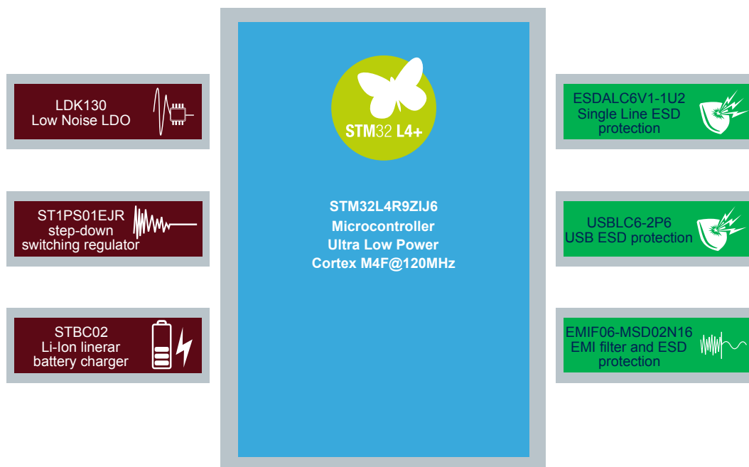
Figure 12. Power and protection components
