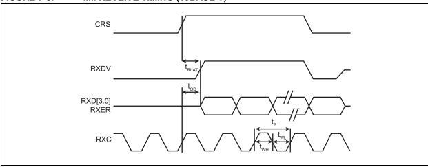
TABLE 7-3: MII RECEIVE TIMING (10BASE-T) PARAMETERS
