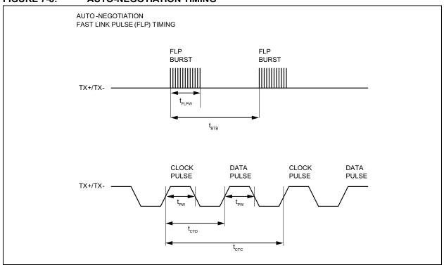
TABLE 7-8: AUTO-NEGOTIATION FAST LINK PULSE (FLP) TIMING PARAMETERS
