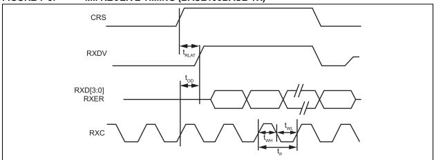
TABLE 7-5: MII RECEIVE TIMING (BASE100BASE-TX) PARAMETERS
