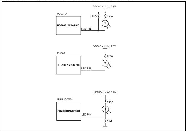
For using 1.8V VDDIO, should select parts with low 1.8V operation voltage and forwarding current IF about 2 mA LED indicator. It is okay to use internal pull-up or external pull-up resistor for the LED pin pull-up strap function, and use an external 0.75 k $\Omega$  to 1 k $\Omega$  pull-down resistor for the LED pin pull-down strap function.
