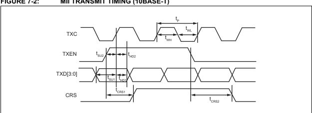
**TABLE 7-2: MII TRANSMIT TIMING (10BASE-T) PARAMETERS**
