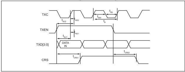
TABLE 7-4: MII TRANSMIT TIMING (BASE100BASE-TX) PARAMETERS
