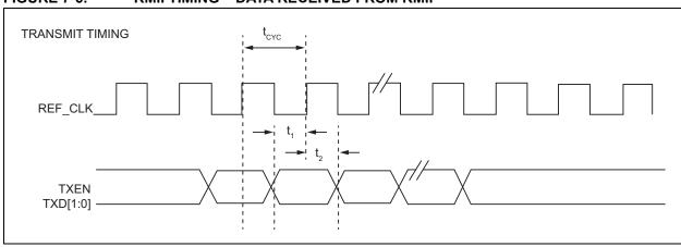
FIGURE 7-7: RMII TIMING – DATA INPUT TO RMII
