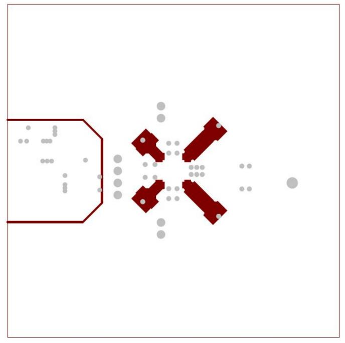
Figure 13. Layer 7 GND Plane
