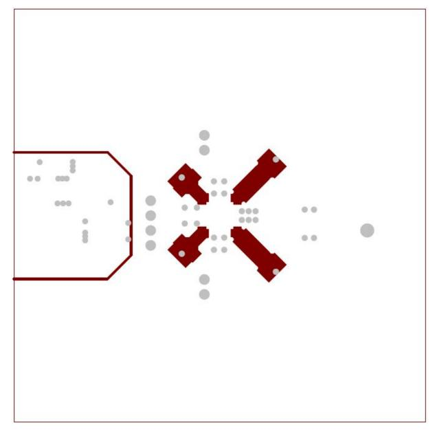
Figure 9. Layer 3 GND Plane
