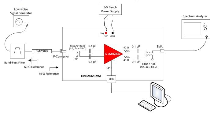
Figure 2. LMH2832 Evaluation Board Setup Block Diagram
