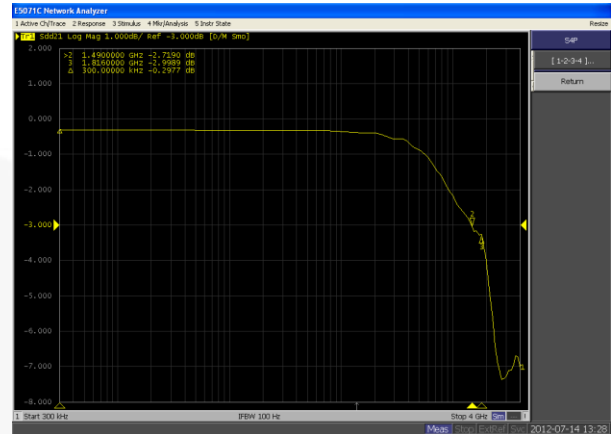
Figure 18. USB Path SDD21 Insertion Loss Curve
