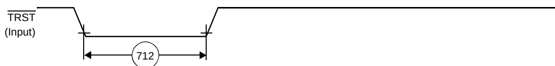
Figure 25. \overline{\text{TRST}} Timing Diagram
