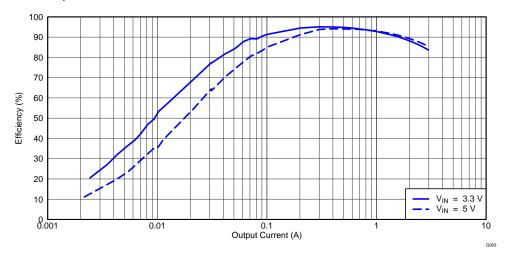
Figure 2. TPS5432EVM-116 Low Current Efficiency
