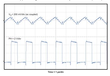
Figure 8. TPS5432EVM-116 Input Ripple
