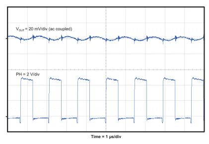
Figure 7. TPS5432EVM-116 Output Ripple
