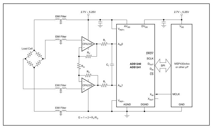
FIGURE 9. Block Diagram for a High-Precision Weigh Scale.
