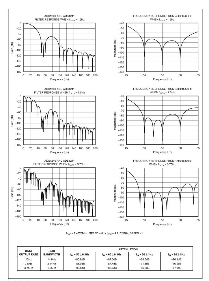
FIGURE 6. Filter Frequency Responses.
