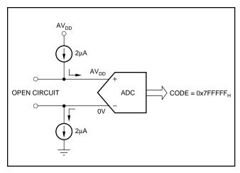
FIGURE 3. Burnout detection while sensor is open-circuited.
