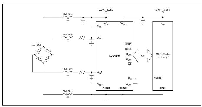
FIGURE 8. Schematic of a General-Purpose Weigh Scale.
