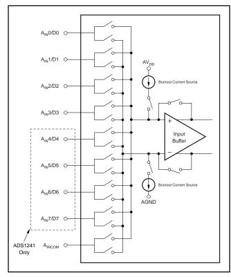
FIGURE 1. Input Multiplexer Configuration.
