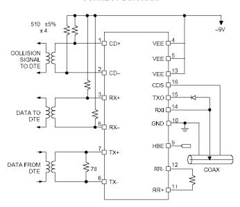
The CD+/- termination resistor may be increased to  $1.5K\Omega$  to save power. Refer to the CD+/- pin description in the data sheet for specific information.
