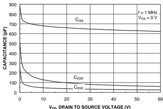
Figure 8. Capacitance Characteristics.
