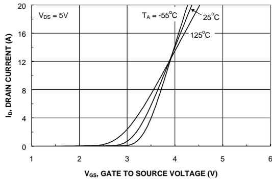
Figure 5. Transfer Characteristics.
