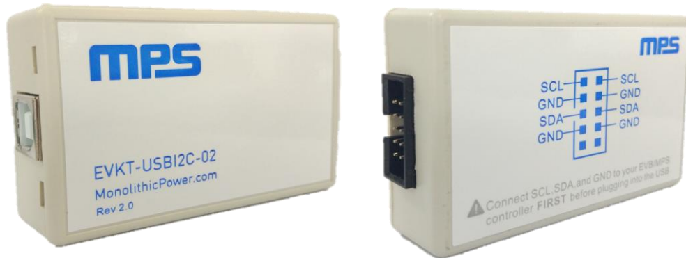
Figure 3: EVKT-USBI2C-02 Communication Interface
