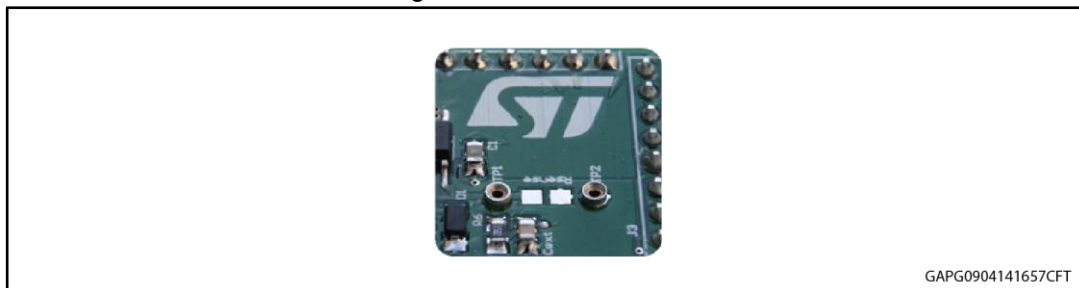
Figure 4: Mounting through-hole sense resistor
