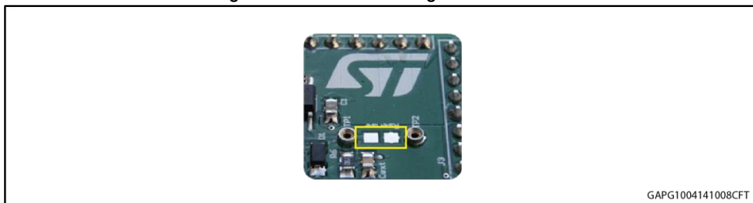
Figure 5: Pads for soldering SMD resistor
