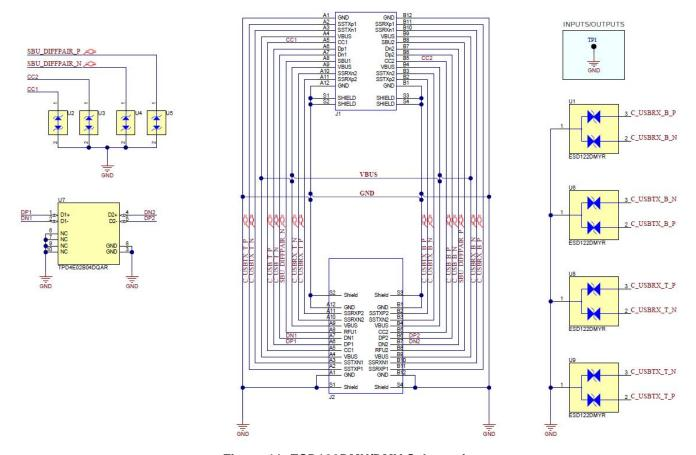
Figure 11. ESD122DMX/DMY Schematic
