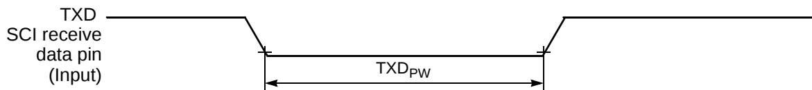
Figure 10-16 TXD Pulse Width
