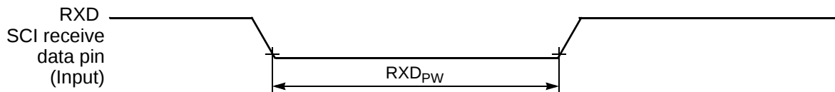
Figure 10-15 RXD Pulse Width
