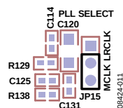
Figure 11. MCLK Loop Filter Selected
