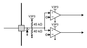
Figure 24. Tri-level Input Pin Diagram
