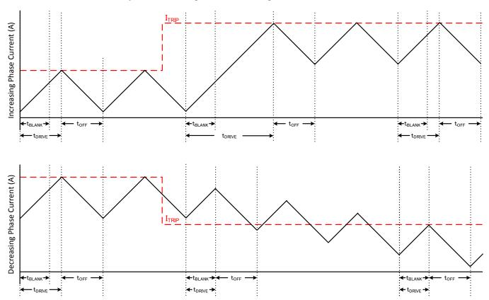
Figure 20. Fast/Fast Decay Mode
