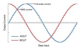
Figure 12. Full-Scale and rms Current
