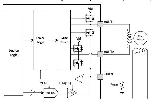
Figure 13. PWM Motor Driver Block Diagram
