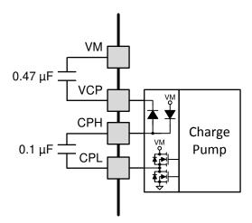
Figure 21. Charge Pump Diagram
