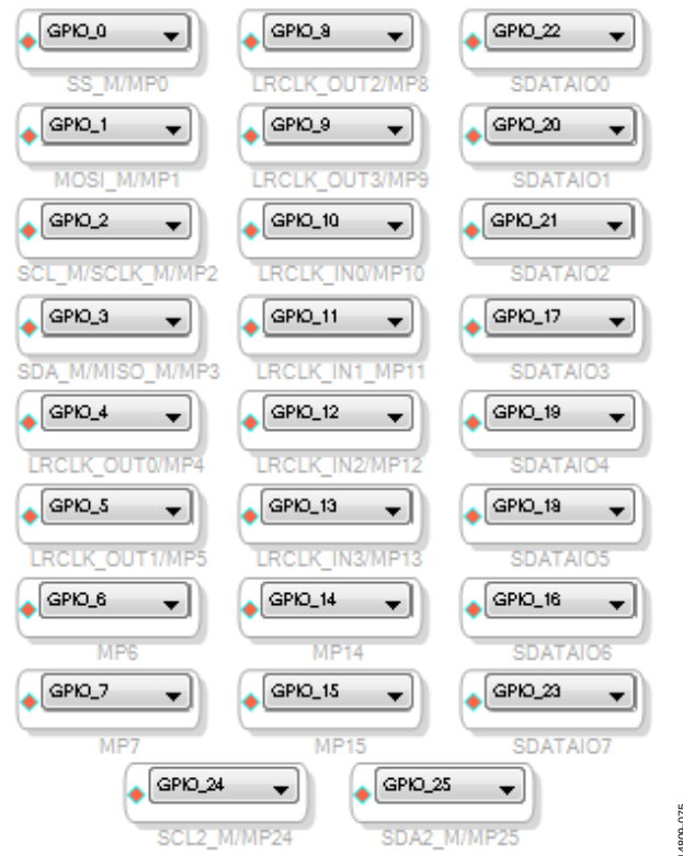
Figure 76. Complete Set of General-Purpose Outputs in SigmaStudio
