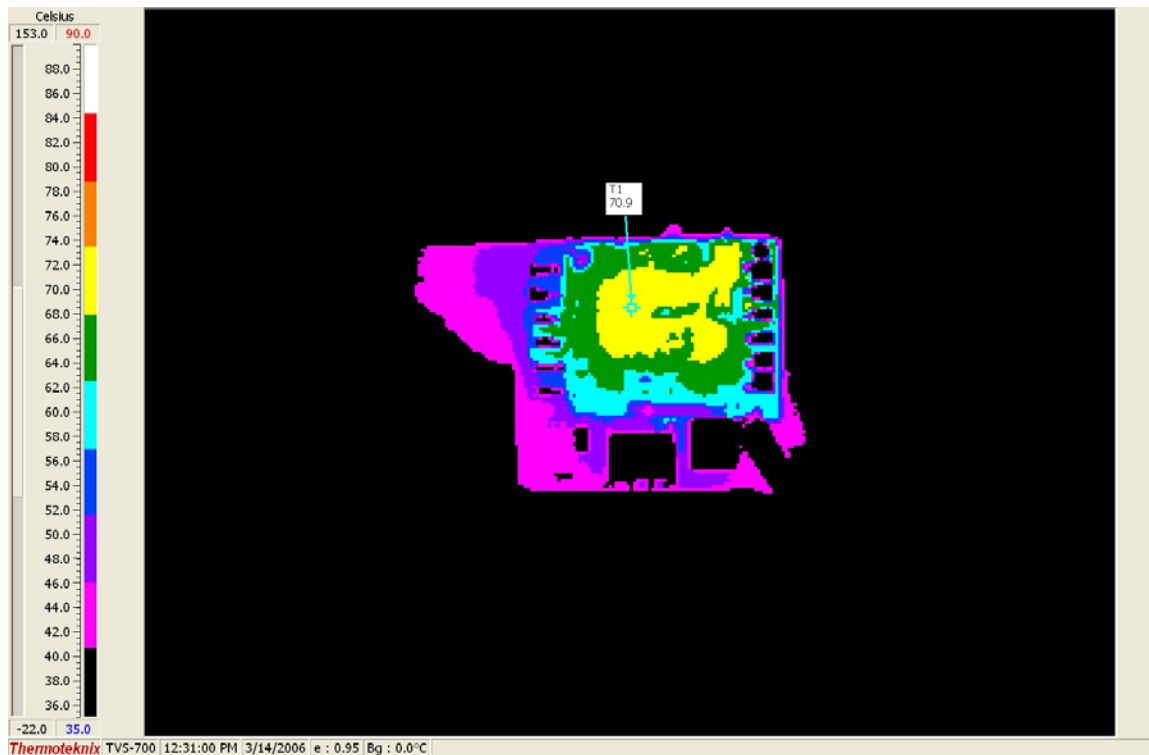
Figure 7. Temp Data (48Vin, 5A, 100LFM airflow – front)
