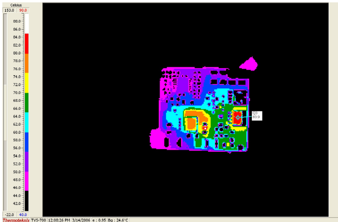
Figure 8. Temp Data (48Vin, 8A, 100LFM airflow – back)
