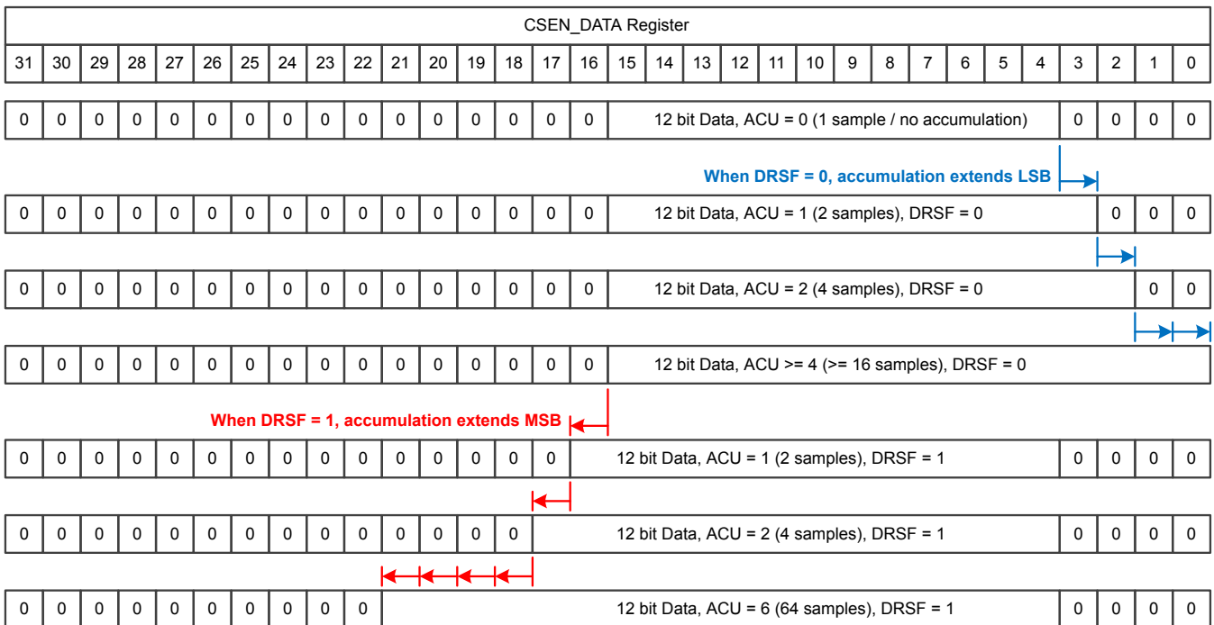
Figure 35.7. Data Encoding for Different Accumulator Settings
