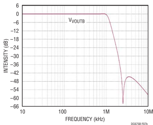
Figure 7. LT1568 Fourth Order Elliptic Lowpass Filter
