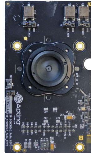
Figure 1. MT9V114 Evaluation Board
