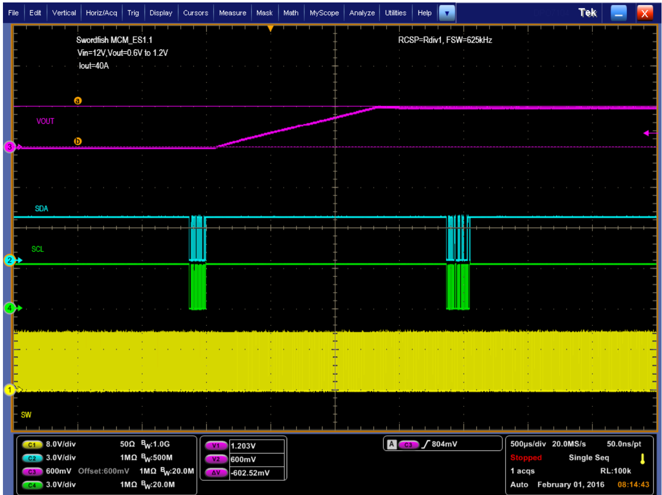
Figure 10. PMBus V OUT Step-Up = 0.6 V to 1.2 V at 40 A
