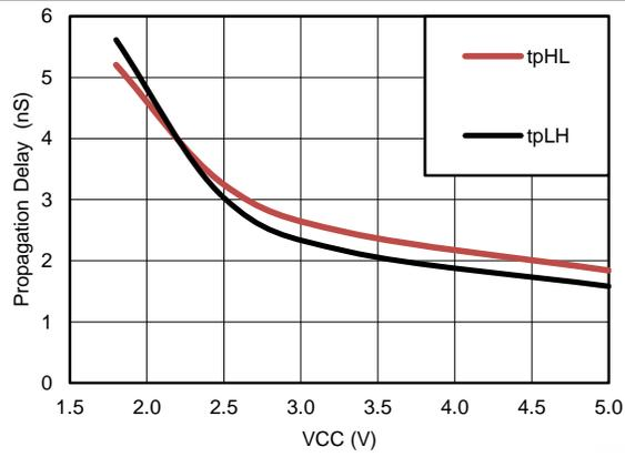
Figure 1. Propagation Delay vs. V<sub>CC</sub>
