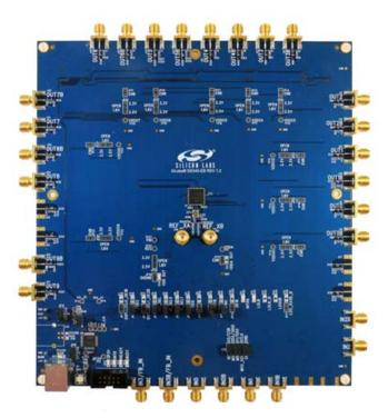
Figure 1. Si5341-D Evaluation Board
