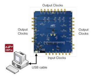
Figure 6. EVB Connection Diagram
