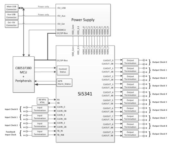
Figure 2. Si5341-D-EB Functional Block Diagram
