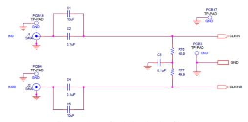
Figure 4. Input Clock Termination Circuit
