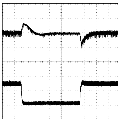
Figure 2. Output Voltage During a Typical Start-Up With a 20V Input and a Load of 150 mA
