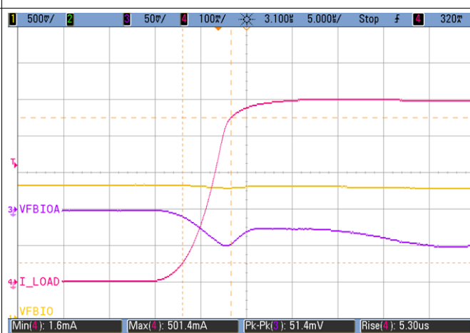
Figure 7-5. VDD2 Rising Load Transient Response
