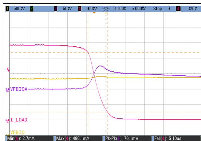
Figure 7-4. VDD2 Falling Load Transient Response
