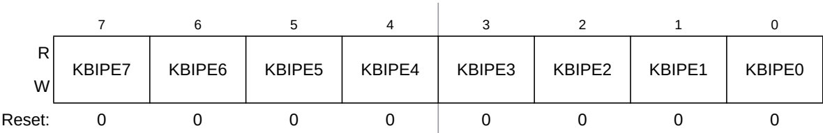
Figure 7-4. KBIX Pin Enable Register
