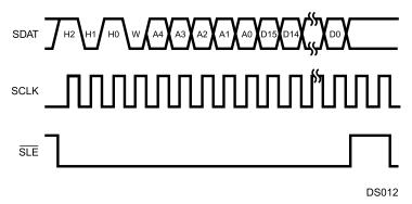
Figure 15-3. Serial Interface Write Timing
