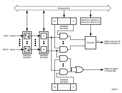
Figure 13-1. Multi-Input Wake-Up Module Block Diagram
