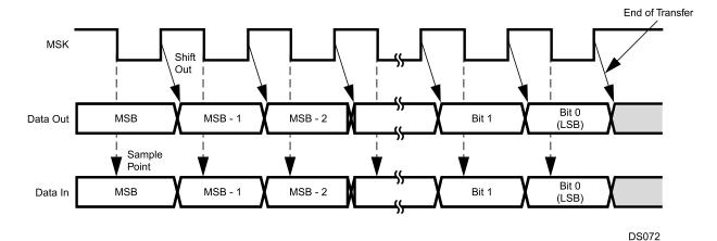
Figure 23-6. Alternate Mode (SCIDL = 1)
