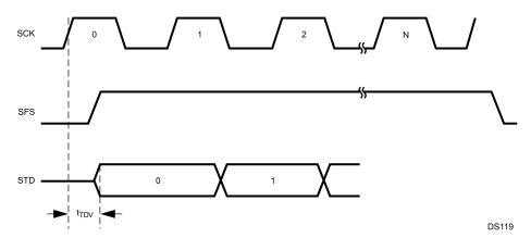
Figure 30-10. Transmit Timing, Long Frame Sync
