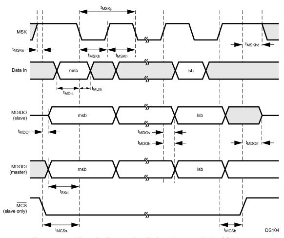
Figure 30-14. Microwire Transaction Timing, Alternate Mode, SCIDL = 1
