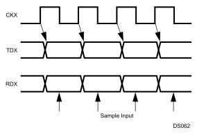
Figure 22-3. UART Synchronous Communication
