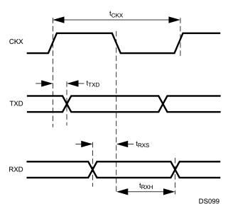
Figure 30-5. UART Synchronous Mode Timing
