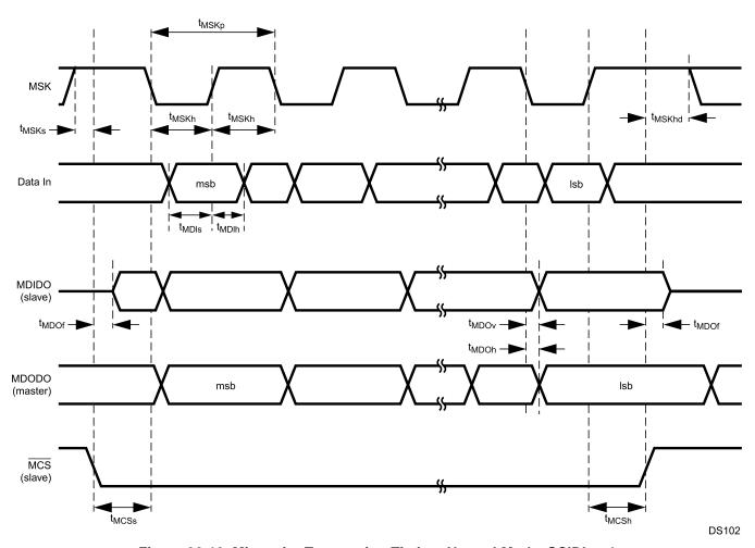
Figure 30-12. Microwire Transaction Timing, Normal Mode, SCIDL = 1
