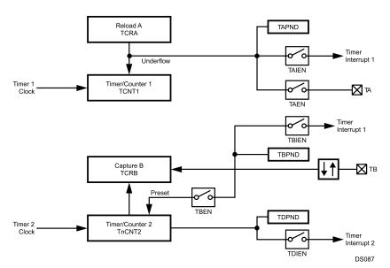
Figure 26-7. Input Capture Plus Timer Mode
