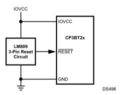
Figure 11-5. Simple External Reset
