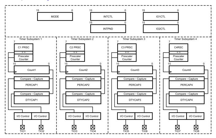
Figure 27-1. Versatile Timer Unit Block Diagram
