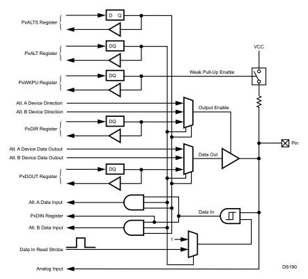
Figure 14-1. I/O Port Pin Logic
