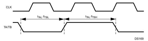
Figure 30-20. Multi-Function Timer Input Timing
