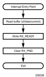
Figure 19-22. Buffer Read Routine (BUFFLOCK Enabled)
