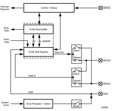
Figure 23-2. Microwire Block Diagram
