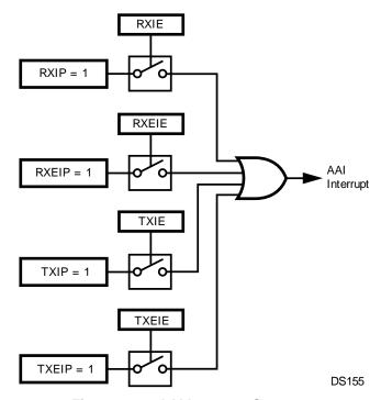
Figure 20-6. AAI Interrupt Structure
