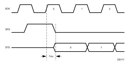
Figure 30-8. Transmit Timing, Short Frame Sync
