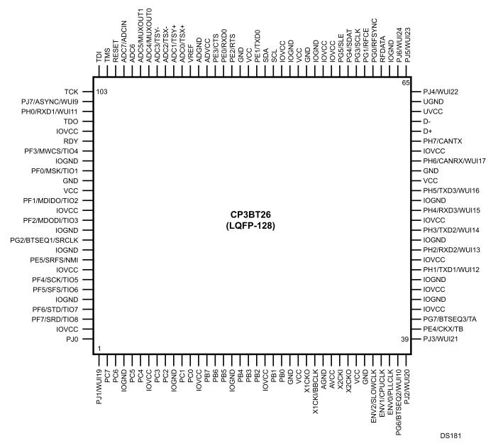
Figure 31-1. CP3BT26 in the LQFP-128 Package (Top View)
