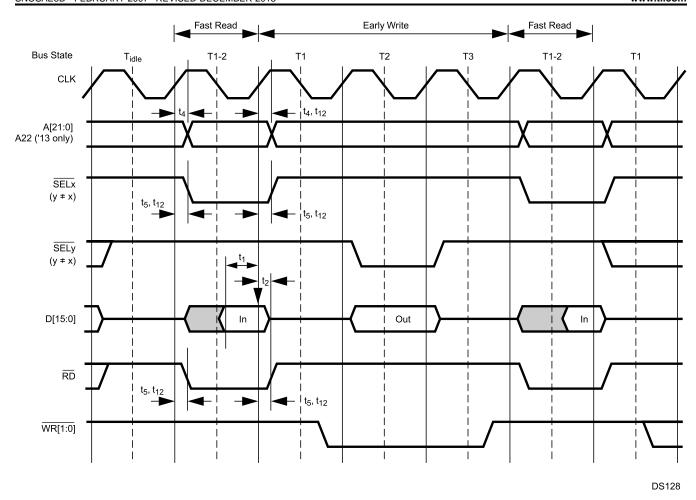
Figure 30-26. Early Write Between Fast Read Cycles
