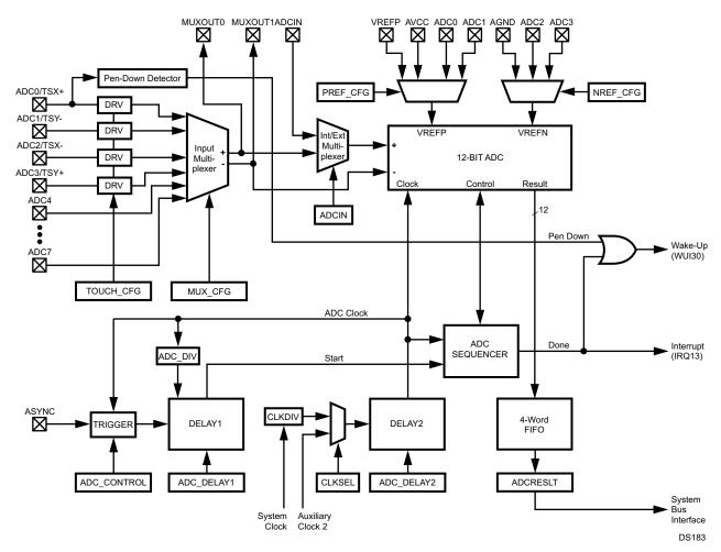
Figure 16-1. Analog to Digital Converter Block Diagram
