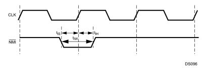
Figure 30-2. NMI Signal Timing
