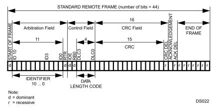
Figure 19-5. Standard Remote Frame
