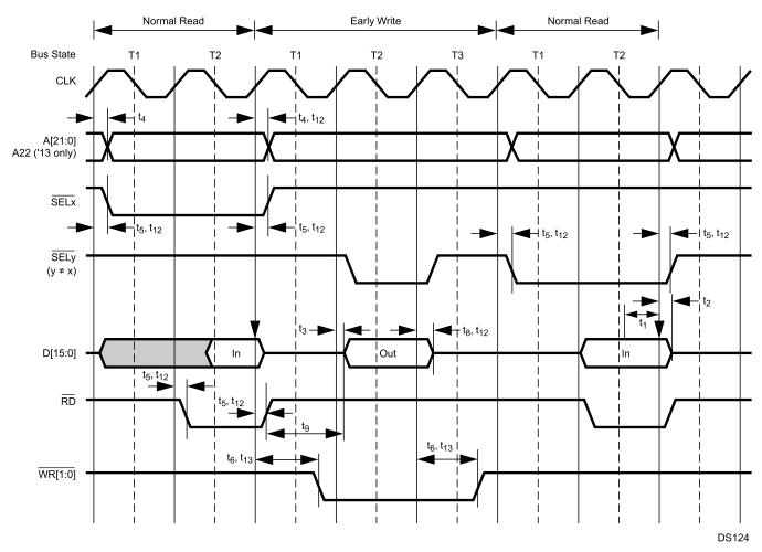
Figure 30-22. Early Write Between Normal Read Cycles (No Wait States)
