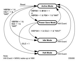
Figure 12-1. Power Mode State Diagram
