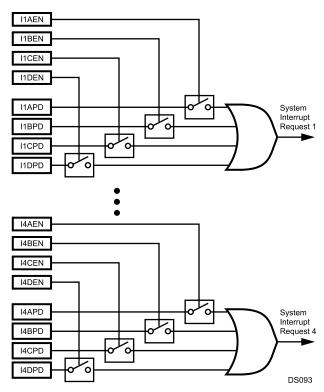
Figure 27-6. VTU Interrupt Request Structure
