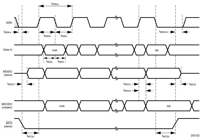
Figure 30-13. Microwire Transaction Timing, Alternate Mode, SCIDL = 0
