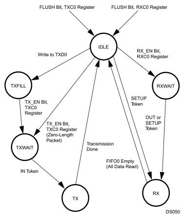
Figure 18-2. Endpoint 0 Operation
