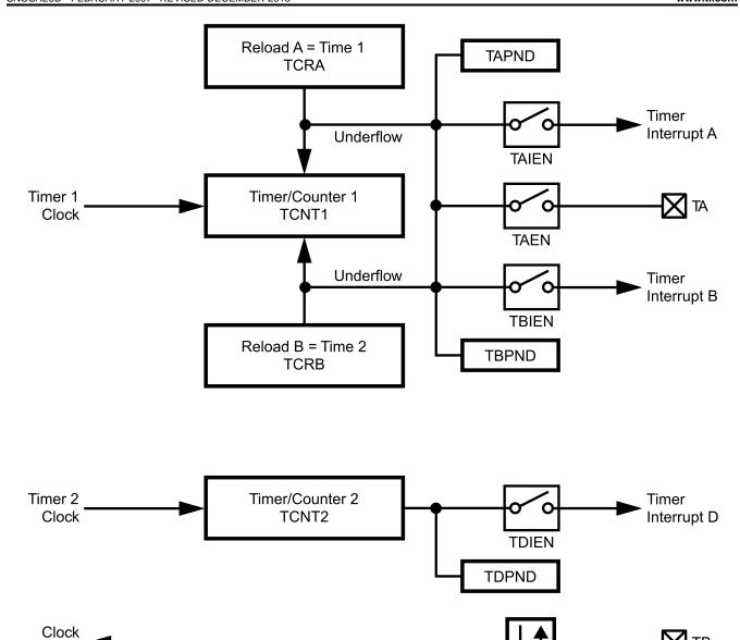
Figure 26-4. Processor-Independent PWM Mode
