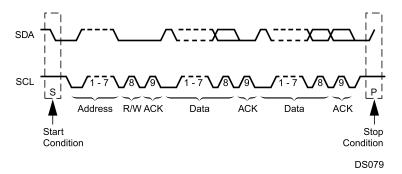
Figure 24-4. A Complete ACCESS.bus Data Transaction
