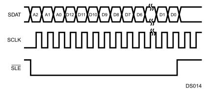
Figure 15-5. Serial Interface 16-bit Fast-Write Timing
