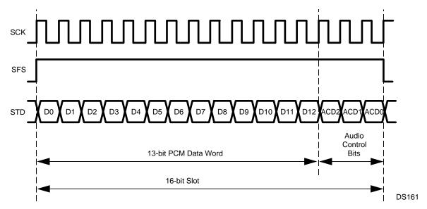
Figure 20-8. Audio Slot with Audio Control Data
