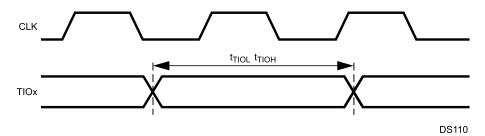
Figure 30-21. Versatile Timing Unit Input Timing
