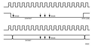
Figure 22-2. UART Asynchronous Communication
