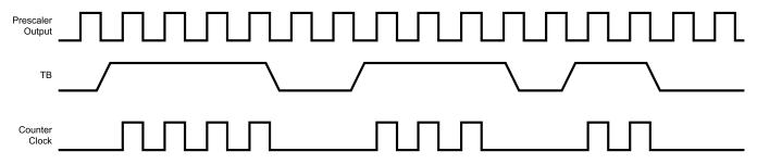
Figure 26-3. Pulse-Accumulate Mode
