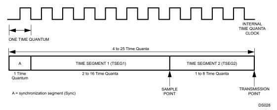
Figure 19-11. Bit Timing
