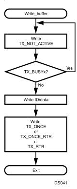
Figure 19-24. Buffer Write Routine
