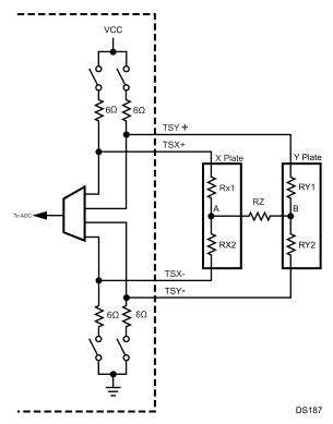
Figure 16-3. Touchscreen Driver Equivalent Circuit
