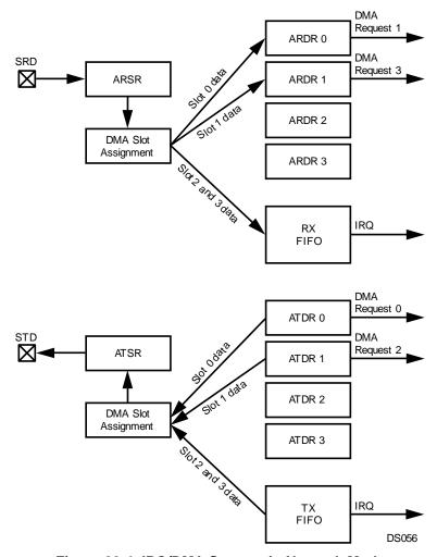
Figure 20-4. IRQ/DMA Support in Network Mode
