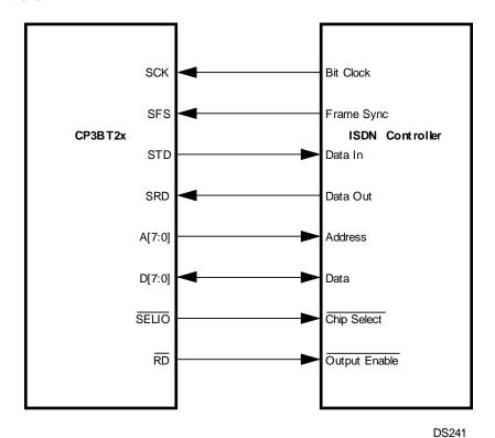
Figure 20-10. CP3BT26/ISDN Controller Connections
