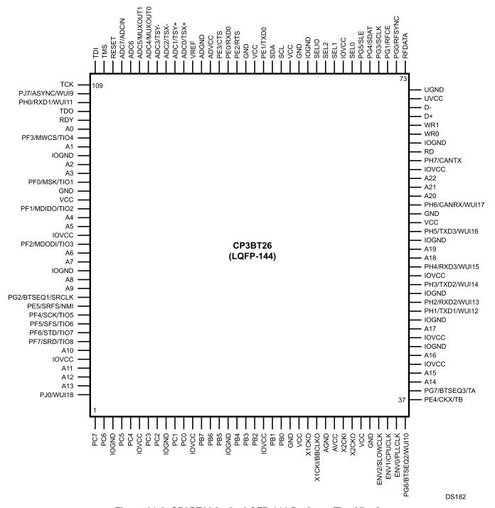
Figure 31-2. CP3BT26 in the LQFP-144 Package (Top View)
