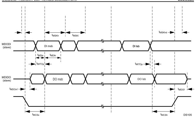
Figure 30-15. Microwire Transaction Timing, Data Echoed to Output, Normal Mode, SCIDL = 0, ECHO = 1, Slave Mode
