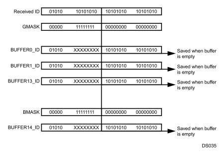
Figure 19-18. Message Storage with BUFFLOCK Enabled
