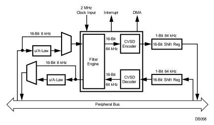
Figure 21-1. CVSD/PCM Converter Block Diagram
