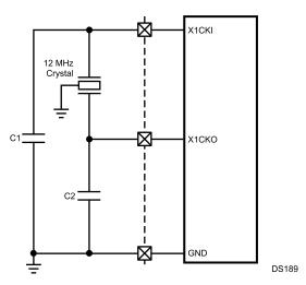
Figure 11-2. Main Clock External Crystal Network
