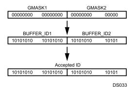
Figure 19-16. Acceptance of a Single Identifier
