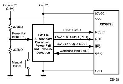
Figure 11-7. Fault-Tolerant External Reset
