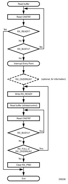
Figure 19-21. Buffer Read Routine (BUFFLOCK Disabled)
