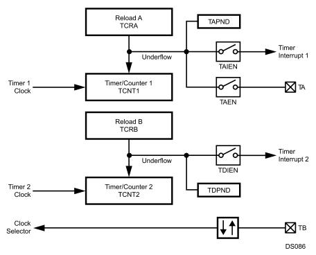
Figure 26-6. Dual-Independent Timer/Counter Mode
