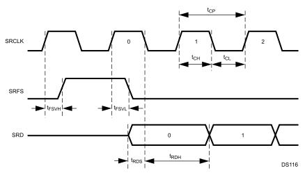
Figure 30-7. Receive Timing, Short Frame Sync
