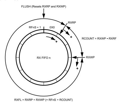
Figure 18-4. Receive FIFO Operation
