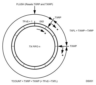
Figure 18-3. Transmit FIFO Operation
