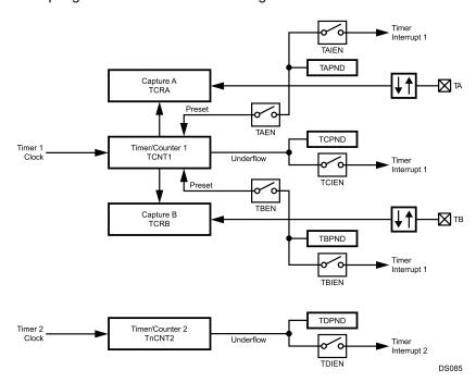
Figure 26-5. Dual-Input Capture Mode
