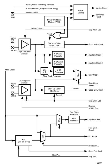
Figure 11-1. Triple Clock and Reset Module
