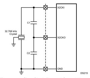
Figure 11-3. Slow Clock External Crystal Network
