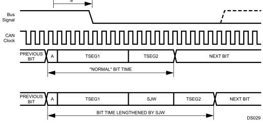
Figure 19-12. Resynchronization (e > SJW)
