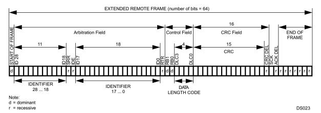
Figure 19-6. Extended Remote Frame
