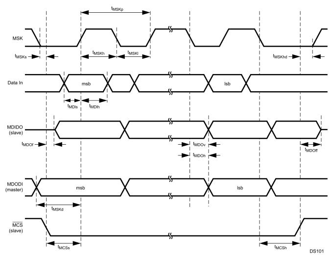
Figure 30-11. Microwire Transaction Timing, Normal Mode, SCIDL = 0
