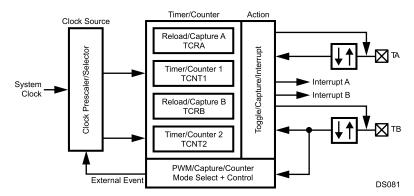
Figure 26-1. Multi-Function Time Block Diagram
