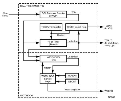
Figure 25-1. Timing and Watchdog Module Block Diagram
