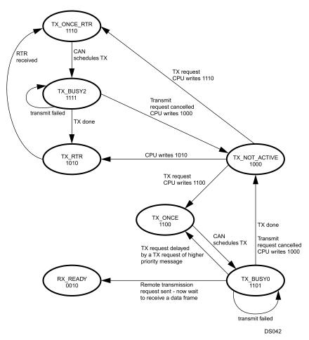
Figure 19-25. Transmit Buffer States
