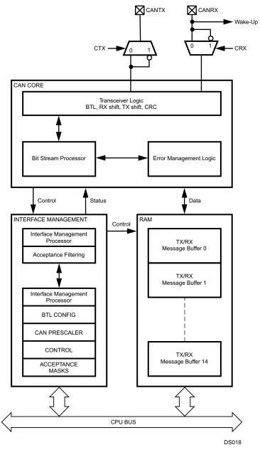
Figure 19-1. CAN Block Diagram
