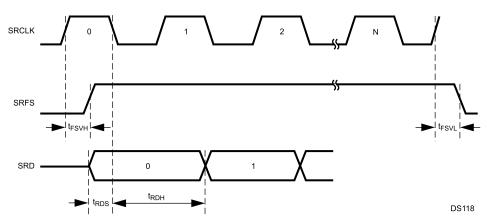
Figure 30-9. Receive Timing, Long Frame Sync
