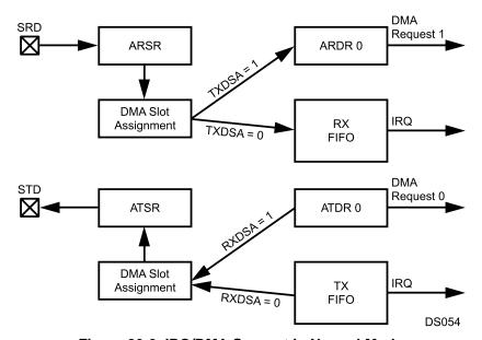
Figure 20-2. IRQ/DMA Support in Normal Mode
