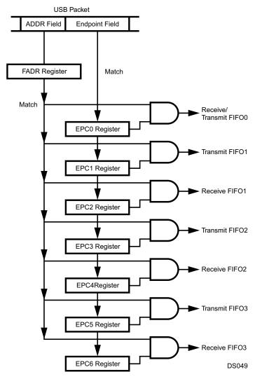
Figure 18-1. USB Function Address/Endpoint Decoding
