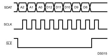
Figure 15-6. Serial Interface 8-bit Fast-Write Timing
