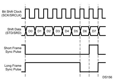
Figure 20-7. Short and Long Frame Sync Pulses
