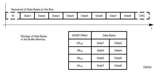
Figure 19-28. Data Direction Bit Clear
