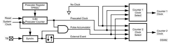
Figure 26-2. Multi-Function Timer Clock Source
