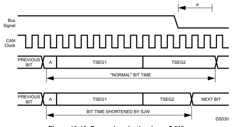
Figure 19-13. Resynchronization (e < - SJW)
