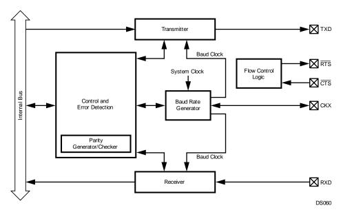
Figure 22-1. UART Block Diagram
