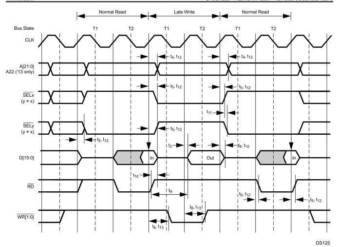
Figure 30-23. Late Write Between Normal Read Cycles (No Wait States)
