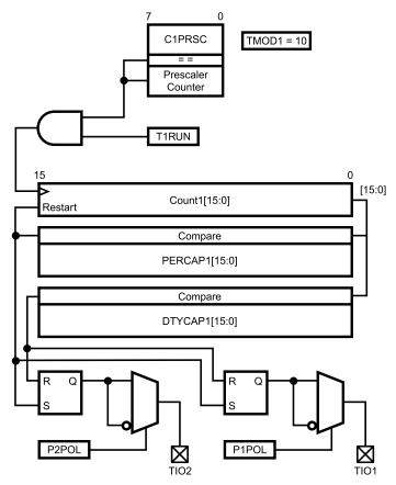
Figure 27-5. VTU Dual 16-bit Capture Mode
