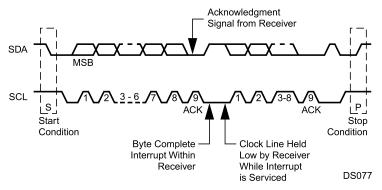
Figure 24-3. ACCESS.bus Data Transaction
