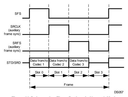
Figure 20-5. Accessing Three Devices in Network Mode
