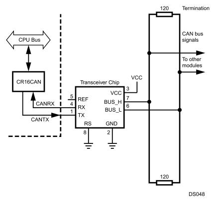
Figure 19-31. External Transceiver
