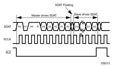
Figure 15-4. Serial Interface Read Timing
