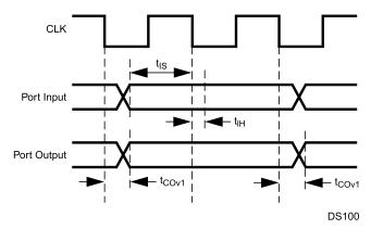
Figure 30-6. I/O Port Timing
