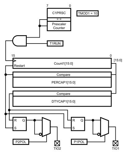
Figure 27-4. VTU 16-bit PWM Mode
