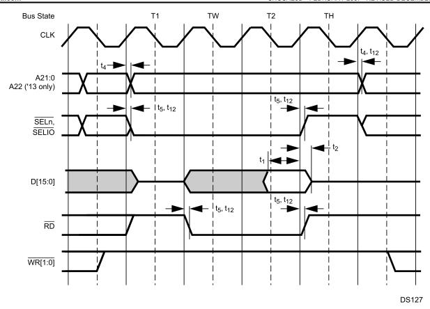
Figure 30-25. Normal Read Cycle (Wait Cycle Followed by Hold Cycle)
