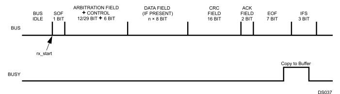
Figure 19-20. Receive Timing
