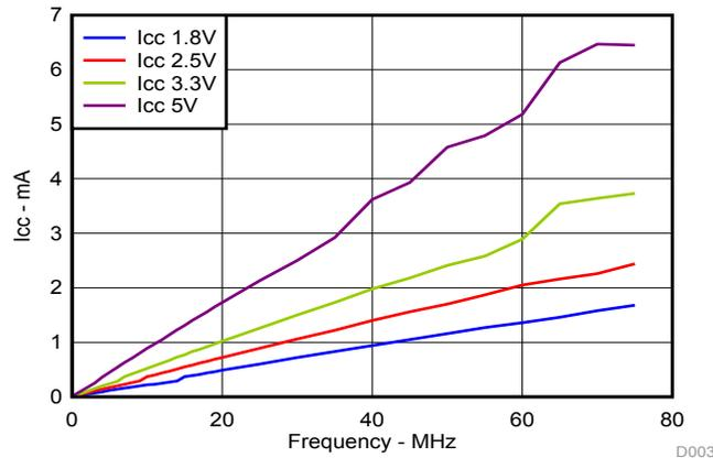
Figure 5. I<sub>CC</sub> vs Frequency
