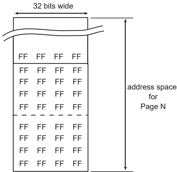
Figure 22-9. Partial Page Programming
