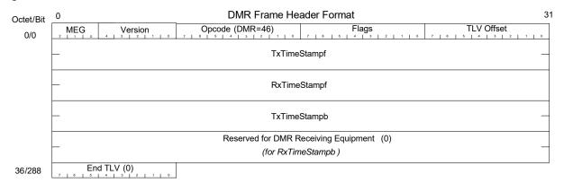
As with PTP, there is no protocol validation for Y.1731 frames; only interpretation of the header to determine what action to take. The first four bytes of the header are used to determine the action to be taken.
