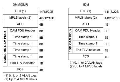
As with PTP, there is no protocol validation for MPLS OAM; only interpretation of the header to determine what action to take. The first four bytes of the header are used to determine the action to be taken.
