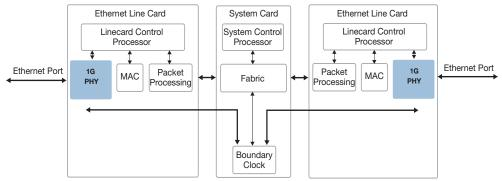
This solution also works for pizza boxes. To ensure that blade redundancy works, it the PHYs for the redundant blades must have the same 1588-in-the-PHY configuration.
