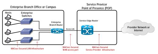
Each host has a dedicated physical link to an Enterprise Ethernet switch, and the switches are connected to an enterprise branch router that also provides WAN access. In smaller configurations, hosts can also connect directly to the branch router. All internal branch office Ethernet ports are secured using MACsec.
