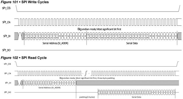
A 25 MHz SPI operating rate is used to access the CSR address space.
