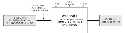
Figure 3 • Fiber Media Transceiver Application Diagram
