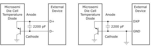
Note: Microsemi does not support or recommend operation of the thermal diode under reverse bias.
