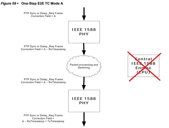
When the system works in one-step E2E TC mode Sync and Delay\_req frames must be forwarded through the system and the residence time = (Egress time stamp – Ingress time stamp) must be added to the correction field in the frame before it leaves the system.
