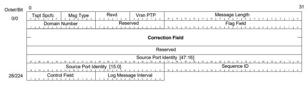
Unlike most of the other stages, there is no protocol validation for PTP frames; only interpretation of the header to determine what action to take. The first eight bytes of the header are used to determine the action to be taken. These match fields in the flow comparison registers with a corresponding set of command registers for each flow.
