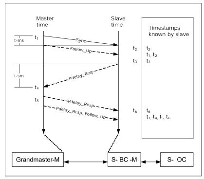
To calculate the path delays on a link, the IEEE 1588 engine (located somewhere in the system) generates Pdelay\_req messages on all ports. When transmitted, the actual Tx time stamp t3 is saved for the CPU to read.
