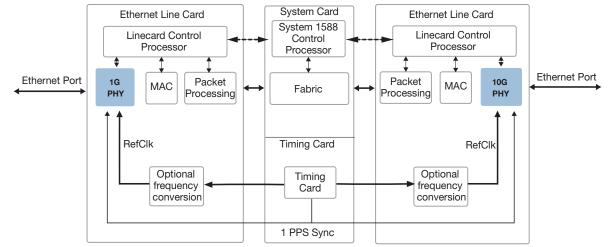
Figure 55 • IEEE 1588 Block Diagram
