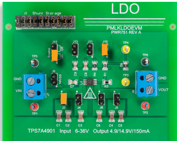
(b) TPS7A4901 LDO regulator operating as dynamic source
