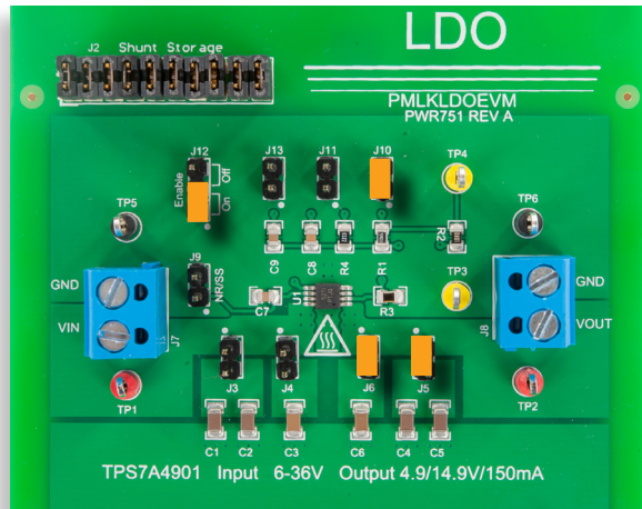
(a) TPS7A4901 LDO regulator under test
