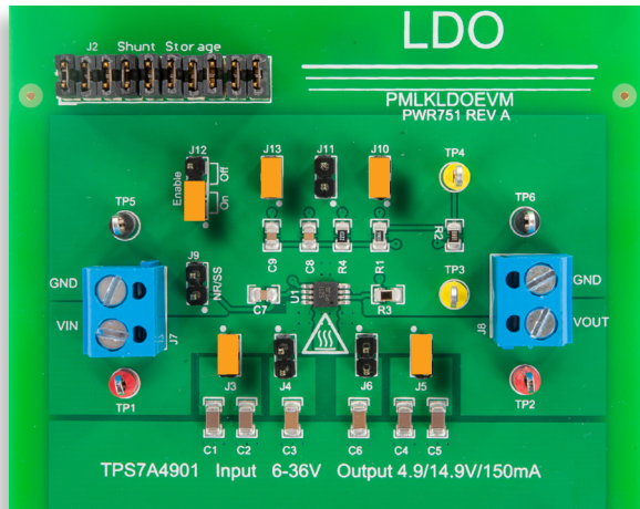
(a) TPS7A4901 LDO regulator under test
