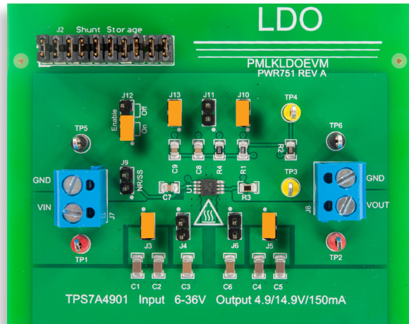
(a) TPS7A4901 LDO regulator under test
