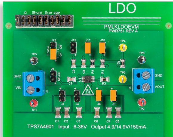
(a) TPS7A4901 LDO regulator under test
