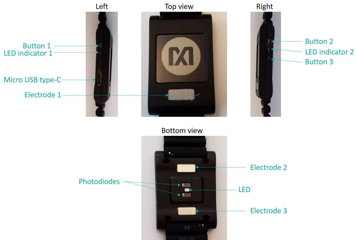
Figure 1. MAXREFDES101# wearable form factor in detail.
