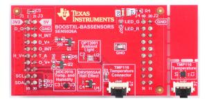
Figure 1. BOOSTXL-BASSENSORS BoosterPack™ Plug-in Module
