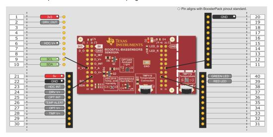
Figure 3. BoosterPack™ Plug-In Module Pinout
