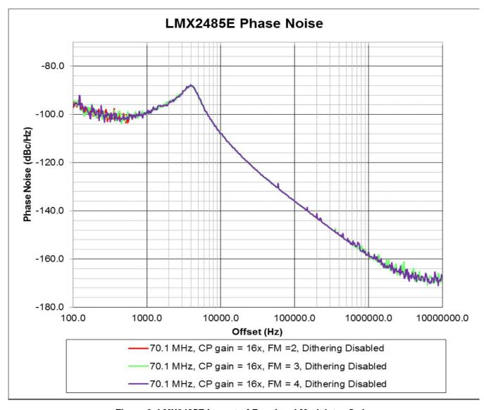
Figure 9. LMX2485E Impact of Fractional Modulator Order
