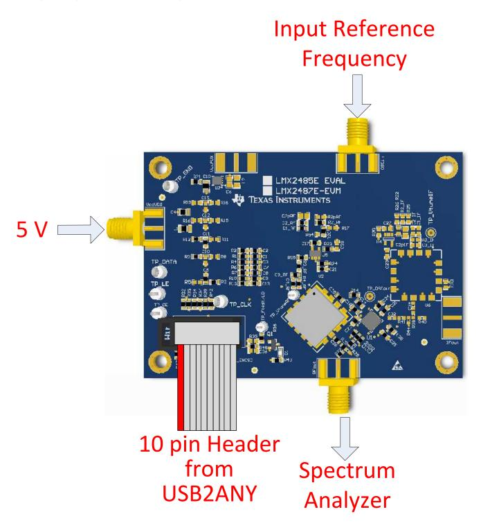
Figure 1. Evaluation Board Setup
