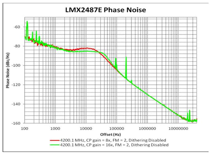
Figure 11. LMX2487E Impact of CPG on Phase Noise
