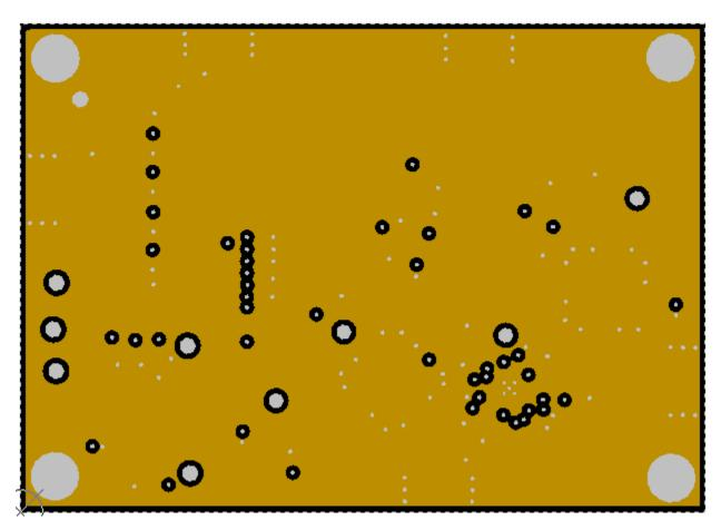
Figure 5. Layer #2 - RF Ground Plane
