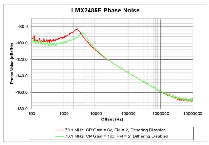
Figure 8. Impact of CPG on Phase Noise
