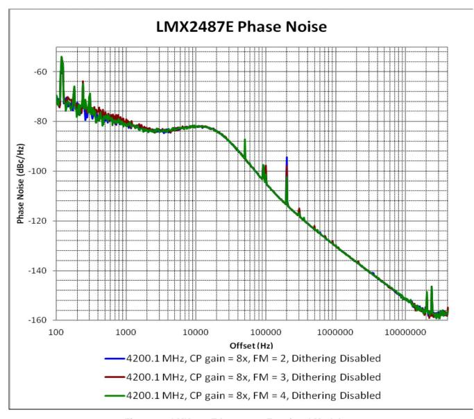
Figure 12. LMX2487E Impact on Fractional Modulator
